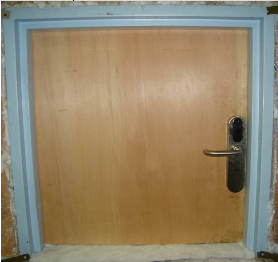
Figure 2 - Typical installation of a Salto XS4 Ei65x Access control furniture on the unexposed side of the door leaf
